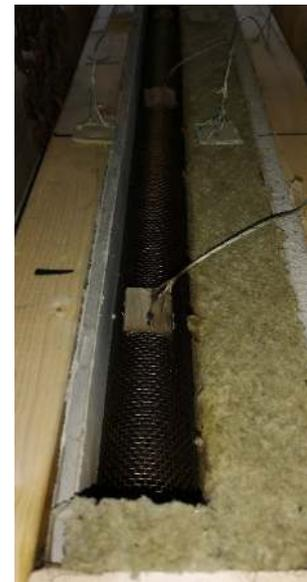
Thermocouples are placed directly on the steel mesh and on both sides of the cavity barrier.
